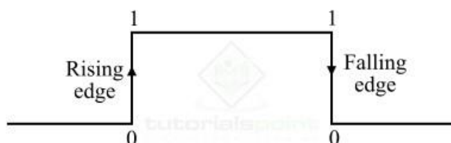
Figure 2 - Clock Pulse Changes State from 0 to 1 or 1 to 0
